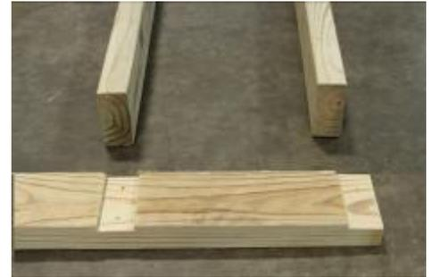
(6) The wider grooves should be placed at the ends.
