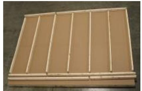
**(25)** Locate and lay out the parts to assemble the back wall.
