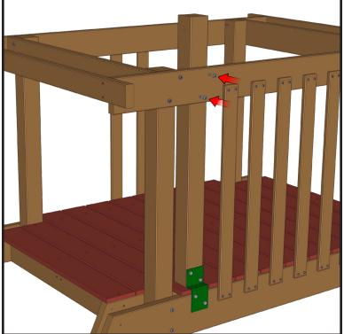
**Step 12.** Fasten the top of the post with two 3" star head lags.
