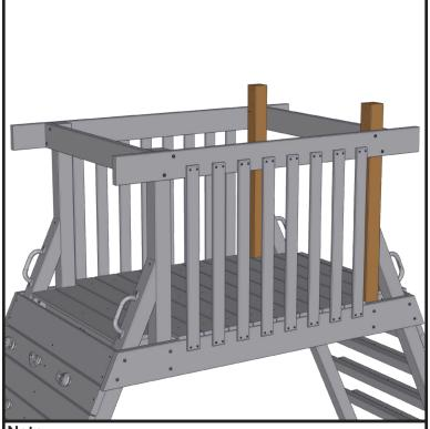
**Note:** If your playset has a space saver swing frame the tower will have two extended 4x4's as shown in the illustration above.
