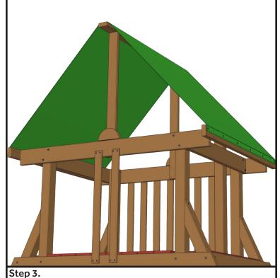
Place the tarp roof over the wood frame and stretch it to fit. Fasten both sides with 1 ¼" washer head screws.
