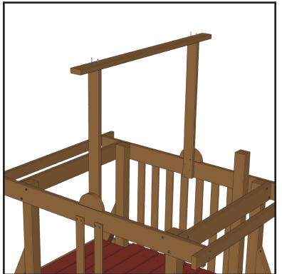
**Step 2.** Place a 59" 2x4 on top of the other 2x4's and center it. Fasten it with 3" wood screws.
