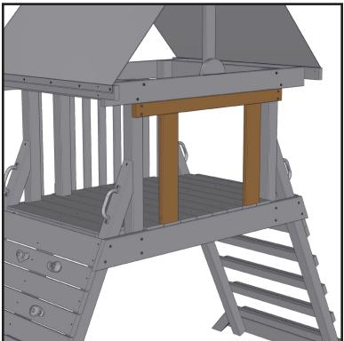
**Sidewinder Slide** Place a 2x4 and two 2x6's in the opening to support the sidewinder slide. Measure the width of the mounting plate on the slide to determine the space between the 2x6's.
