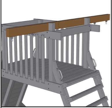
**Step 3.** Place the swing frame on the tower against the inside of the extended 4x4 posts.
