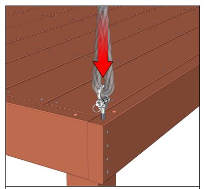
**Step 5.** Each rope assembly has a mounting bolt attached.
