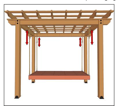
**Step 9.** Tighten all four ropes until the bed is level then remove the support legs to allow the bed to hang freely.
