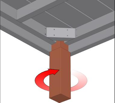
**Step 4.**Rotate each leg 180° and slide back into place.
